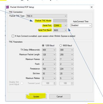
If your TNC is using a serial port or is connected via USB, set the Serial Port. Click the box and Winlink will show you a COM port number. If two or more COMs are shown go to "Device Manager" in Windows and find the correct one. Or just try one...if it fails...pick the other! The Serial Port Baud is set to 9600 by default. You may need to change this based on the radio or TNC you chose in the TNC Type. Use 9600 Baud if unsure. Click Update at the bottom of the window.
