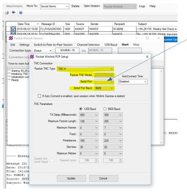
Packet TNC Type. This drop down menu shows the TNC's that have been tested by Winlink creators. If you see your TNC in the list, choose it. MCARA/ARES is using TNC-X as our standard. If you have a TNC and it is not in the list, begin testing using TAPR TNC2. If that fails try KISS.
