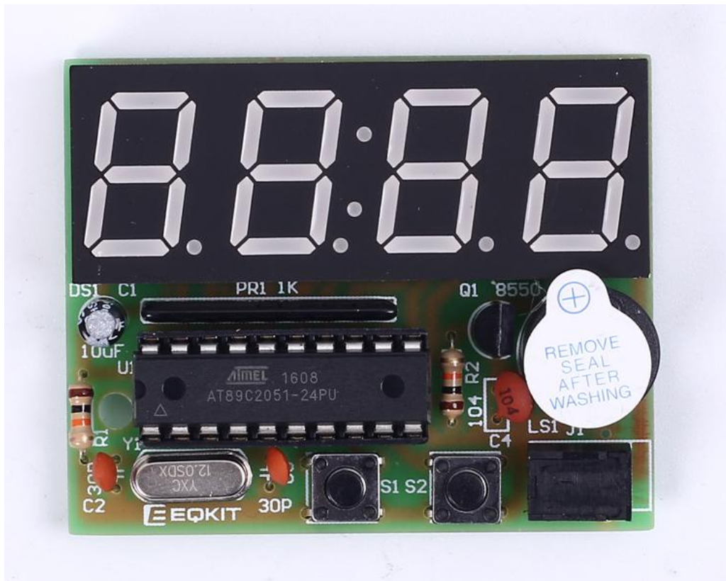
Step 6: Install 4Bit Digital Tube and IC.And then test!
