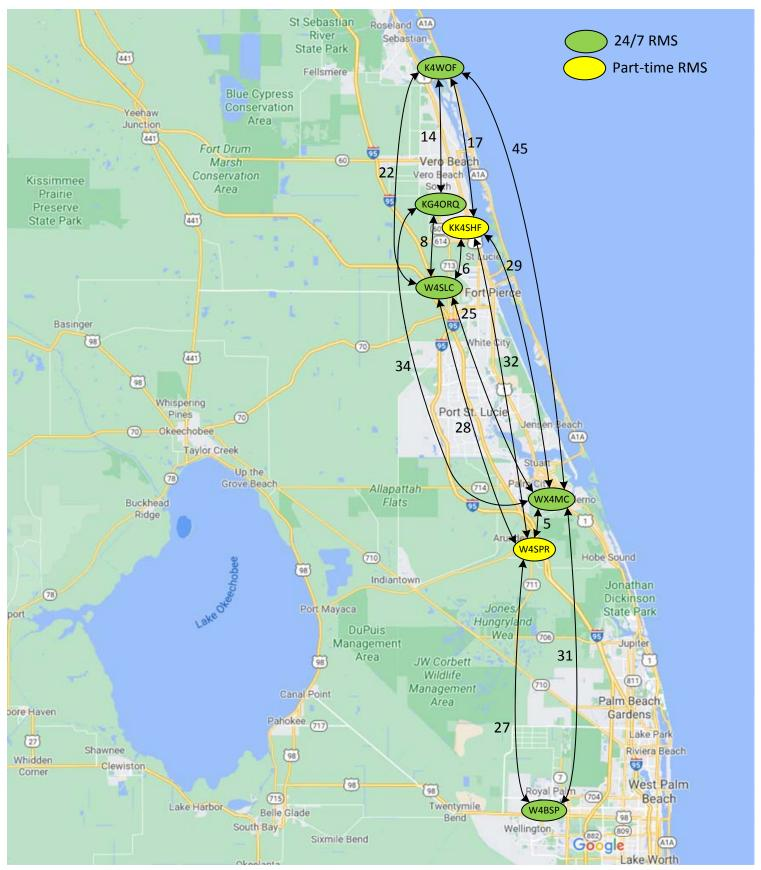
Station to station distances are shown in statute miles, and indicate tested, reliable communication links with existing equipment, running VARA-FM v4.0.1.
